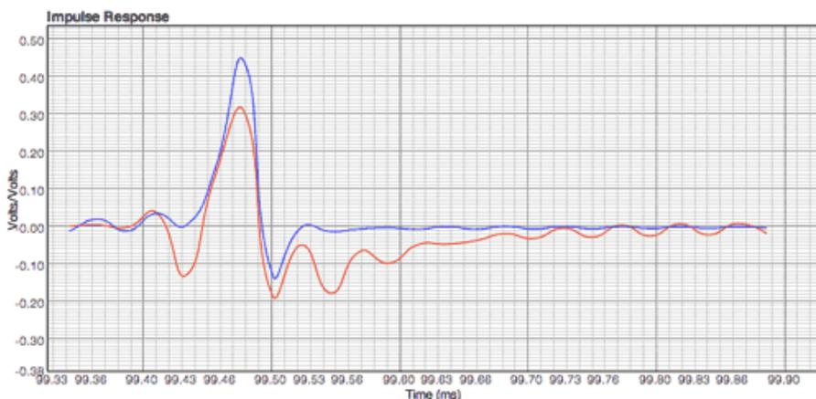
The impulse response of the 5G looks almost perfect, with only a small ripple. The impulse response of the 6G shows misalignment of frequency components; it takes a while before it settles compared to the 5G. This misalignment is reflected by the group delay, which can be deduced from the steepness of the phase response curves. The following figure shows the phase response of the 5G and 6G (due to the measurement grid I can't completely align the phase response).
