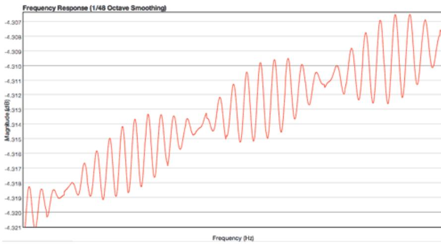
At 1/48th octave smoothing of the curves, there is no sign of such a modulation for the 5G at all. The 6G shows a comb due to the smoothing. With no curve smoothing applied, things start looking worse for both, but especially for the 6G :
